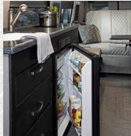
3.5 cubic foot 12v/110v refrigerator with freezer
